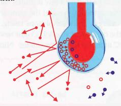
Energy transfers by conduction from the glass molecules to the alcohol molecules inside the bulb. Kinetic energy transfers throughout the alcohol by conduction collisions between alcohol molecules.
