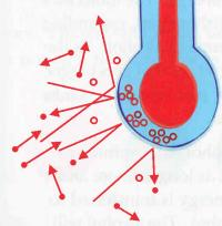
Kinetic energy transfers by conduction from molecule to molecule in the glass bulb until all of the glass molecules are warm.
