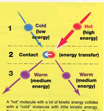
A "hot" molecule with a lot of kinetic energy collides with a "cold" molecule with little kinetic energy. Energy transfers at the point of contact. The cold molecule then has more energy, and the hot molecule has less energy.
